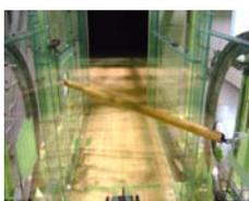
(a) Test view of test of yawed cylinder
