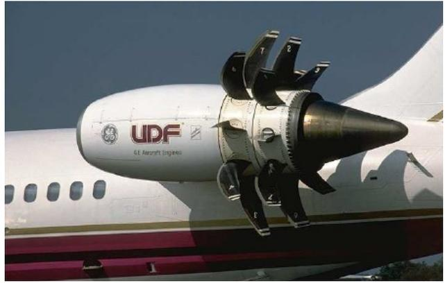
**FIGURE 1:** GENERAL ELECTRIC GE-36 UDF MOUNTED ON A MCDONELL-DOUGLAS MD-80 [4].
