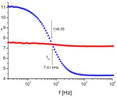
DF frequency mixture with  $\Delta n$ =0.1-0.3 and  $f_{co}$ =3-10 kHz at 20°C have been created. They have similar response times  $\tau_{on}$ - $\tau_{off}$  and the total  $\tau_{on}$ + $\tau_{off}$ < 1ms for applied voltage below 20 V. Examples of prepared LCMs for DF addressing will be presented in details.
