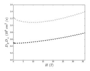
Dependence of the diffusion coefficients of photons  $D_{\parallel}(x)$  and  $D_{\perp}(\blacktriangle)$  on the magnetic field.
