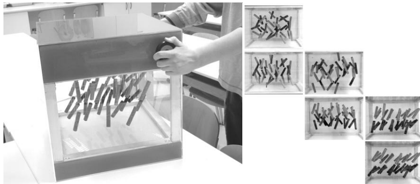
Fig. 1: From left to right: a mechanical model of liquid crystal; phase transitions: isotropic \rightarrow nematic, nematic \rightarrow smectic-A, smectic-A \rightarrow smectic-C.
